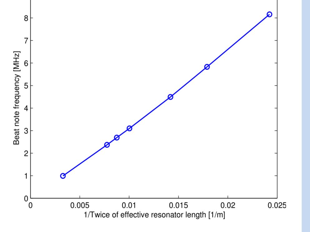
• The comb line spacing depends on the resonator length, with a relation of c/2L, where c is the speed of light, L is the effective resonator length (including the refraction index of the optical fiber).
