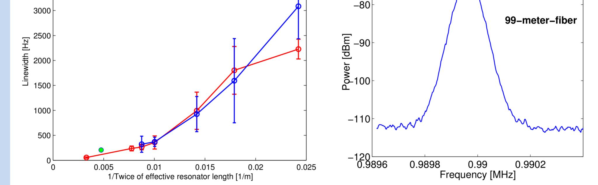
• (A) The self beat linewidth is measured when the output of PCR hits on the photodiode. The comb heterodyne linewidth is when the output of PCR is sent to beat with a reference comb as shown in the section 4. The reference comb is with self beat linewidth of 200Hz (the green dot). (B) The example of self beat linewidth when the resonators consists of a 99 meter fiber. The linewidth is 55Hz, which is much smaller than the situations for the shorter fibers, as shown in the red line in (A).
